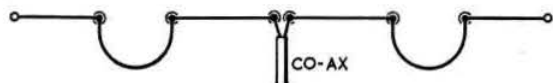
Fig. 1. Shortened 7 Mc/s aerial which could not be made to function on 3.5 Mc/s.
